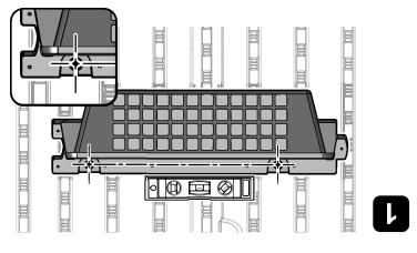
Using a level, a marker and your shed accessory as a template, position and mark wall anchor pilot hole locations. Use the EZ Bolt holes on your accessory as a guide.
