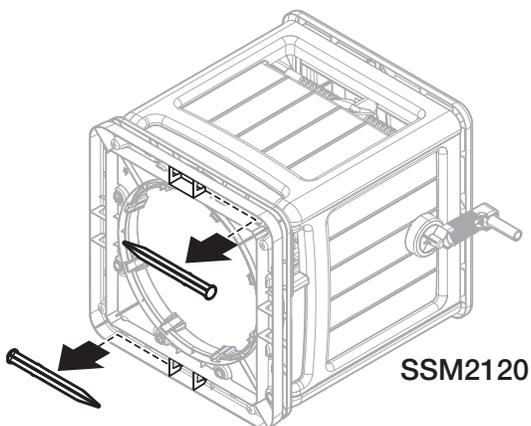
Remove provided stakes from the underside of base. Insert 2 stakes through openings. Secure with rubber mallet.
