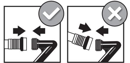
Connect leader hose to the in-tube (A) on the exterior of the hose reel. Connect the opposite end of the leader hose to the water supply.
